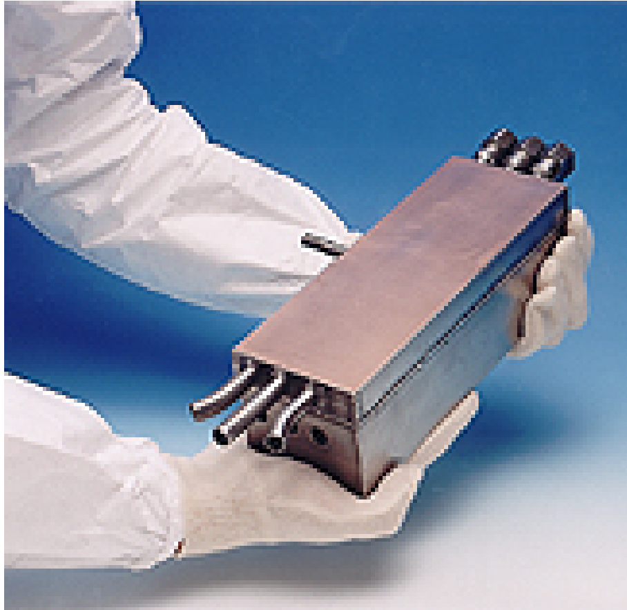
Blanket prototype prior to beryllium tile bonding
