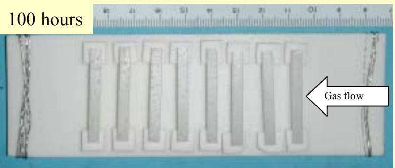
Appearance of the MGC specimens after hot corrosion test
