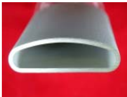
Cross-section diagram of the plasma sprayed mold at the middle of the longitudinal direction
