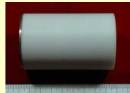
\text{Al}_2\text{O}_3/\text{GAP} rod ( \Phi 53 mm)
