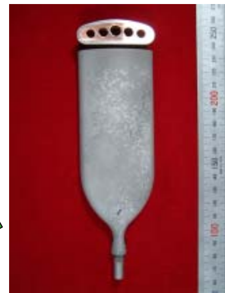
A plasma sprayed mold on a quasi-turbine nozzle copper model
