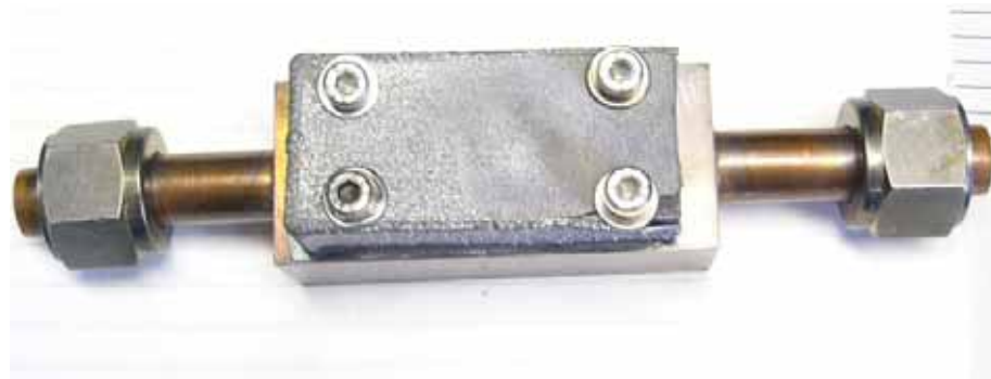
CVD-W coating on graphite ( Re as a interlayer)
