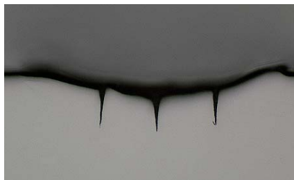
Quantitative analysis of plastic zones around crack-tips in tungsten (picture: UOXFORD)
