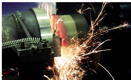
Friction and wear tests of short fibre C/SiC for high power brake applications (picture: MERL)
