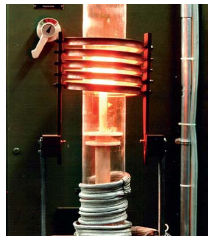
Re-entry tests of new heat shield materials for future European space shuttles (picture: FZJ)
